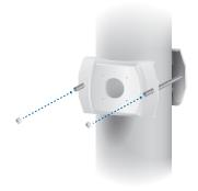
3. Position the camera in front of the appropriate *Mounting Bracket*. Then feed the cable through the opening.
