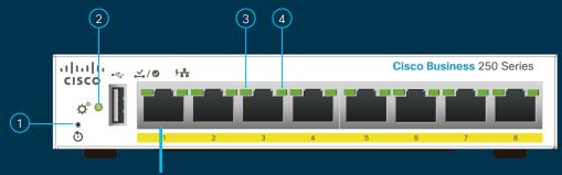
NOTE: On the CBS250-8T-D model, port 1 can work as a PoE PD or PoE input port to power the switch.
