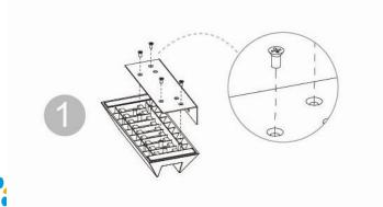
Remove the screws on the stand. The screw the clump weight to the stand again to the stand as the picture shows.
