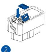
Figure 4 Device case removal
