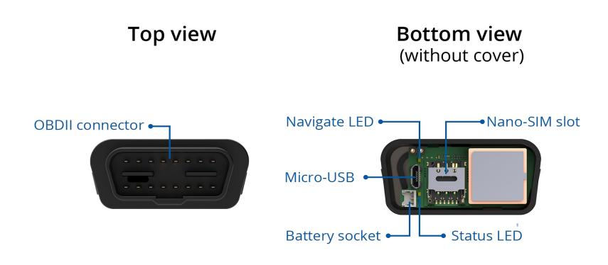
Figure 1 FMB020 device view
