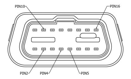
Figure 2 FMB020 OBDII socket pinout
