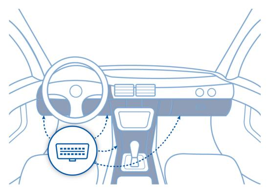
Figure 10. Most common OBDII connector locations.
