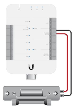
Fail-secure lock in this diagram refers to electric strike.
