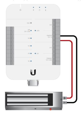
Fail-safe lock in this diagram refers to magnetic lock or electric bolt.
