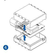
Figure 6 Attaching cover back
