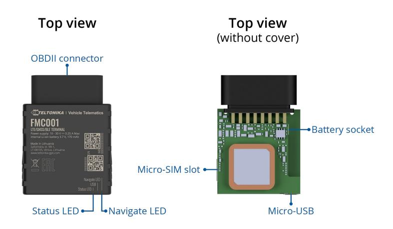
Figure 1 FMC001 device view
