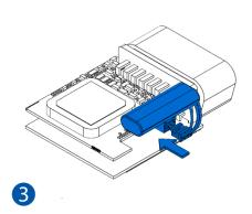
**Figure 5 Battery connection**
