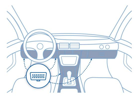
Figure 10. Most common OBDII connector locations.
