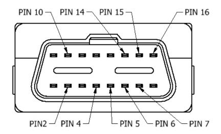
Figure 2 FMC001 OBDII socket pinout
