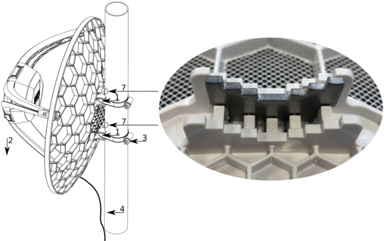
1. Slide the included metallic mounting rings into the two slots on the back of the antenna dish.
