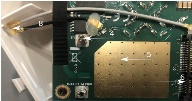
5. Attach provided a thick thermal pad to the card, and install the card into miniPCIe slot so that thermal pad is between PCB and card;
