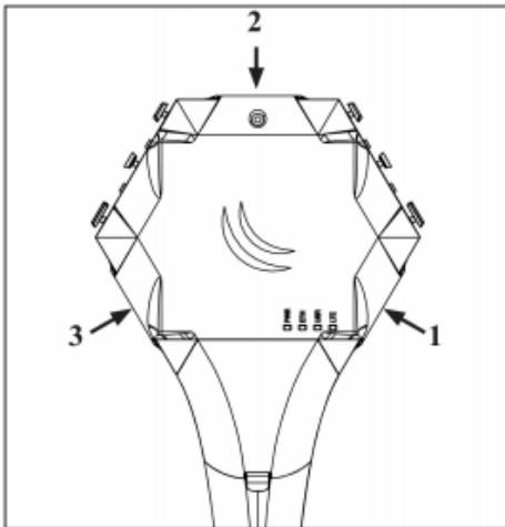
2. Insert a screwdriver into the first slot.
