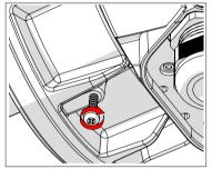
Tighten the locking screw to secure the TwisPort™ lock mechanism.
