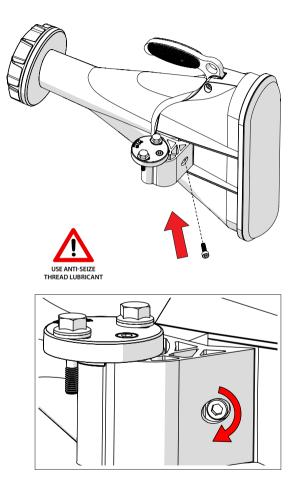
Model HG3-TP-A60 shown. Installation instructions are identical for other Asymmetrical Horn models. Antenna dimensions may differ.
