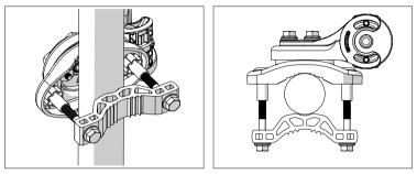
Place the AH-TP Bracket like this for pole diameter of 36 - 49mm
