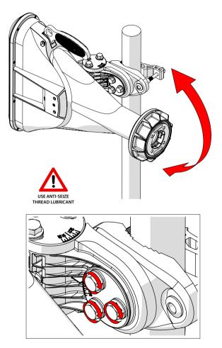
Model HG3-TP-A60 shown. Installation instructions are identical for other Asymmetrical Horn models. Antenna dimensions may differ.
