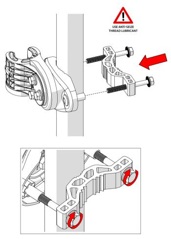
Model HG3-TP-A60 shown. Installation instructions are identical for other Asymmetrical Horn models. Antenna dimensions may differ.
