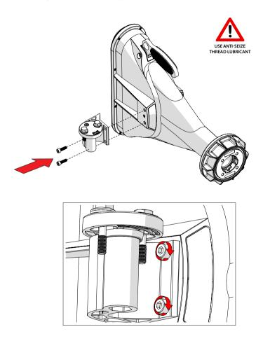
Model HG3-TP-A60 shown. Installation instructions are identical for other Asymmetrical Horn models. Antenna dimensions may differ.
