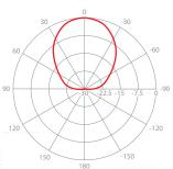
V/H - Port Pattern Azimuth 5.6 GHz
