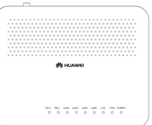
Silk Screen Name **Status** Indication Green: always The device is powered on. on Power supply **POWER** The device is powered by the Orange: always LED backup battery. on 0ff The power supply is cut off. Authentication See Table 4. PON LED LOS Connection LED | See Table 4.
