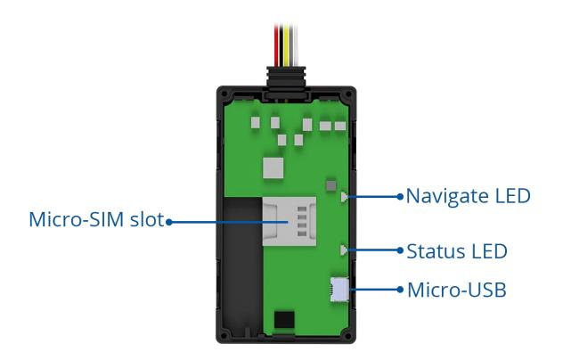
Figure 1 FMB900 device view
