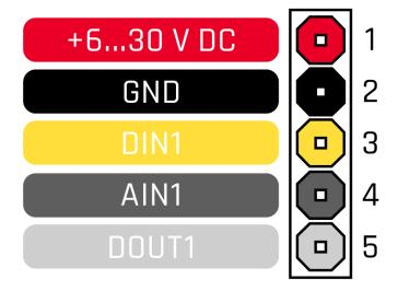
Figure 2 FMB900 pinout
