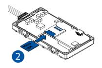
Figure 5 Micro-SIM card insert
