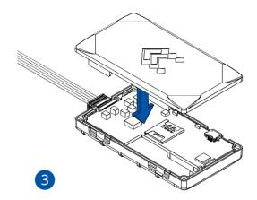
Figure 6 Attaching cover back
