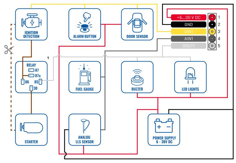
Figure 3 FMB900 Wiring scheme
