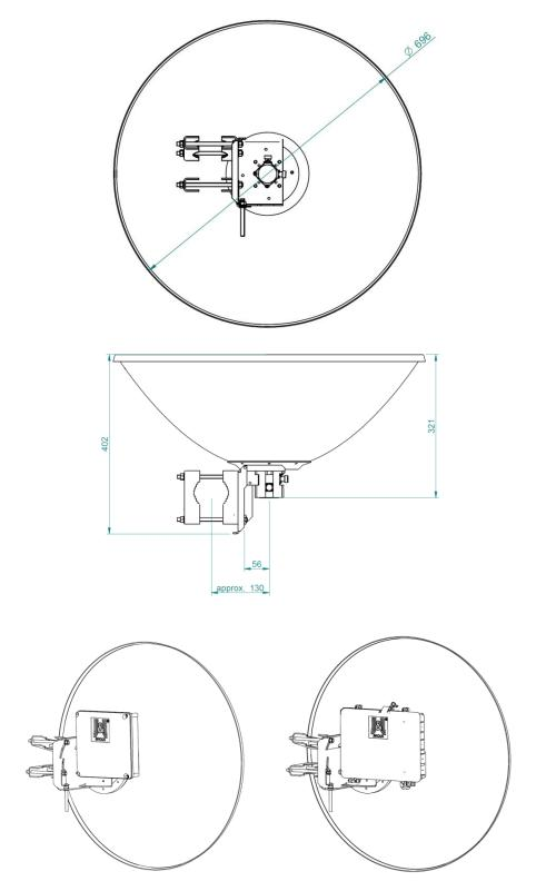
Accessories: outdoor plastic box JR - 200 or metal box JR - 250 Alu - right side mounting only, polarization 45° not possible
