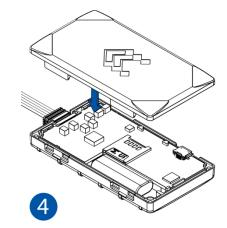
Figure 7 Attaching cover back
