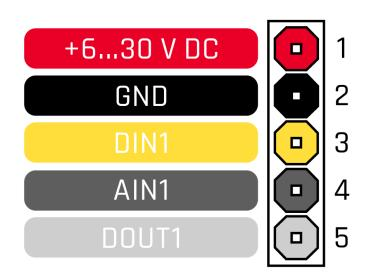
Figure 2 FMB920 pinout
