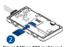
Figure 5 Micro-SIM card insert
