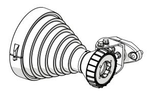
Ensure that the water drain points downwards!
