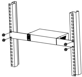
Figure 11 Mounting the Switch on a Rack (ES1100-24)
