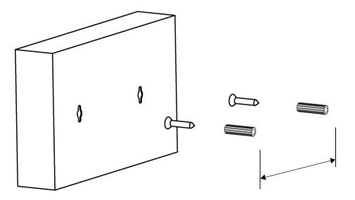
Wall-mount the Switch with the Ethernet ports facing down and the ventilation holes on the side.
